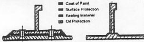
Fig.27 Joint design of A380 passenger cargo (Airbus) 30)
